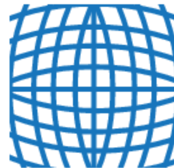
Positive radial distortion "barrel"
